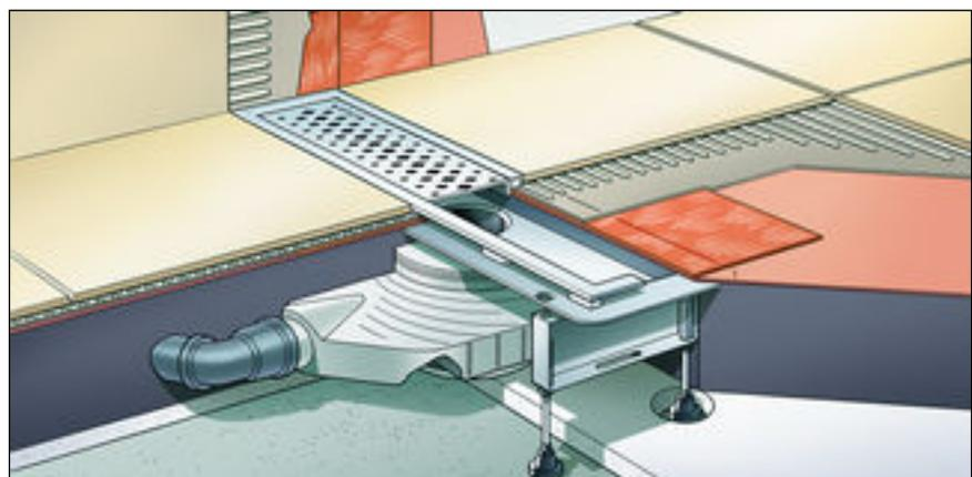
Fig. 2: Diagram of a bonded seal
