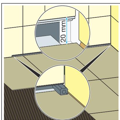
**INFO!** The gap for the standing grate must be exactly 20 mm. Use the tile protection tool and control tool to define the gap size.
