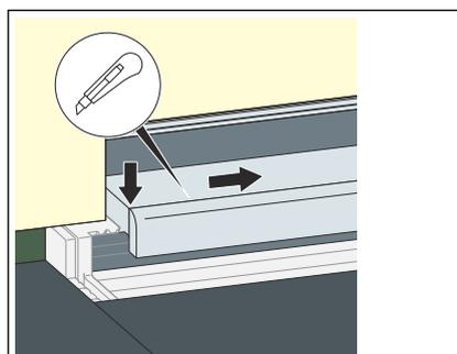
► Remove the front edge of the protective insert.
