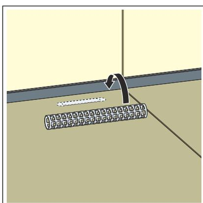
➤ Insert the sieve above the drain in the channel gap.
