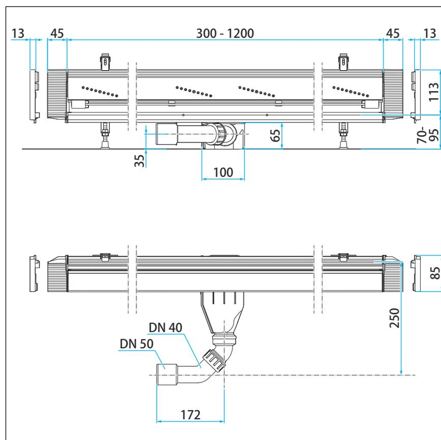
Fig. 17: Dimensions of base unit basic model
