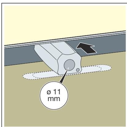
**NOTICE!** Risk of damage during cleaning! To protect the shower channel and the tiles, use the tile protection and checking tool comprised in the delivery.
