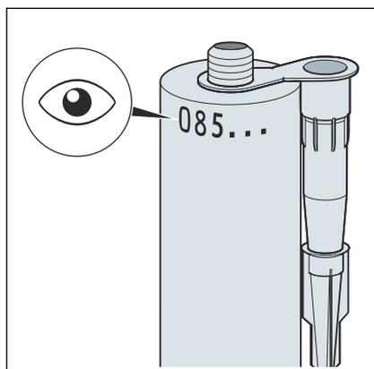
Fig. 16: Filling date of the mounting adhesive
