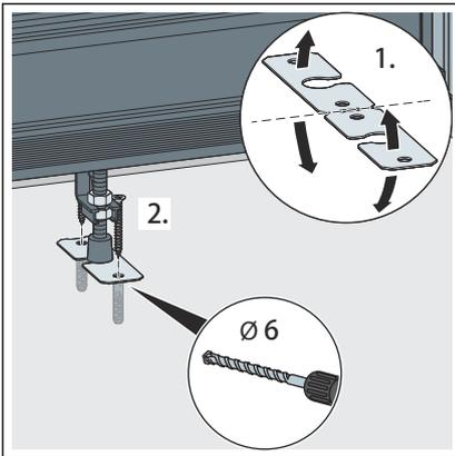
► Secure the feet in place with fixing material if necessary.
