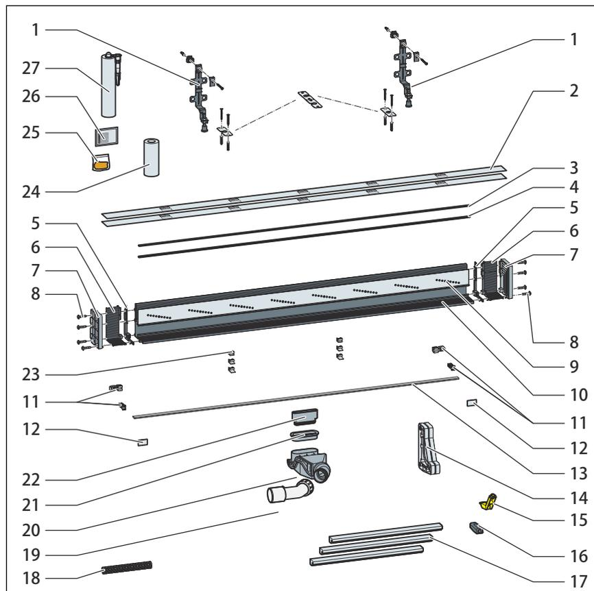
Fig. 12: Components and scope of delivery
