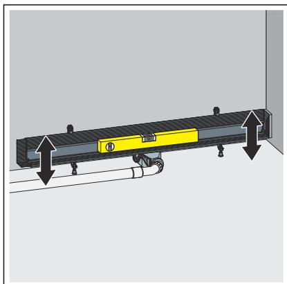
➤ Align the shower channel with the adjustable feet horizontally in all directions.
