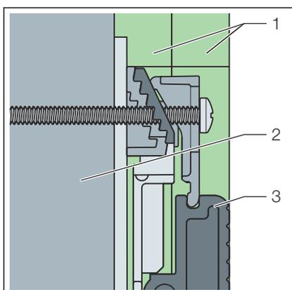
**With two gypsum plaster boards (12.5 mm each)**
