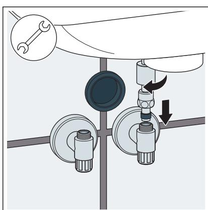
► Push the cover, the fixing screw and the sealing element onto the connection pipe.
