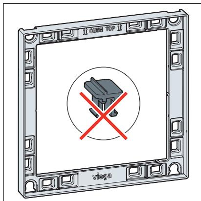
**INFO!** The arrangement of the clips differ according to the flush plate.
