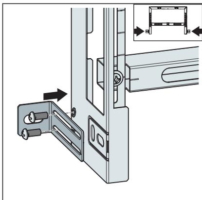
► Screw the metal angles to the bidet block.
