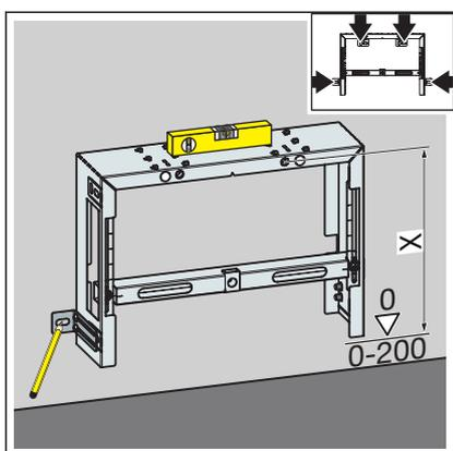
► Adjust the construction height of the bidet block in accordance with the on-site marking of the upper edge of the finished floor.
