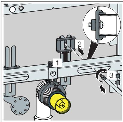
► Mount the mounting bracket for the wall plates.
