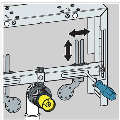
► Adjust the height and width of the mounting bracket.
