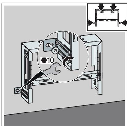
► Tighten the bidet block via the mounting brackets using a fork spanner (size 10).
