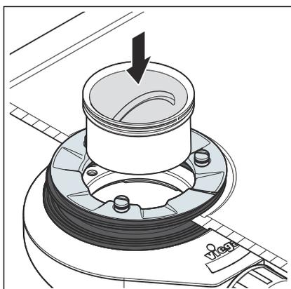
► Insert the immersion pipe into the odour trap.
