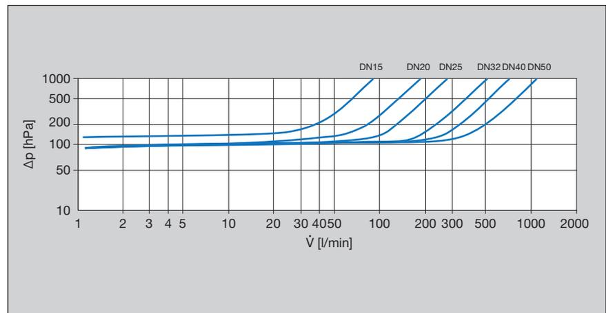
Fig. 1: Performance diagram pressure loss CRV press/threaded connection
