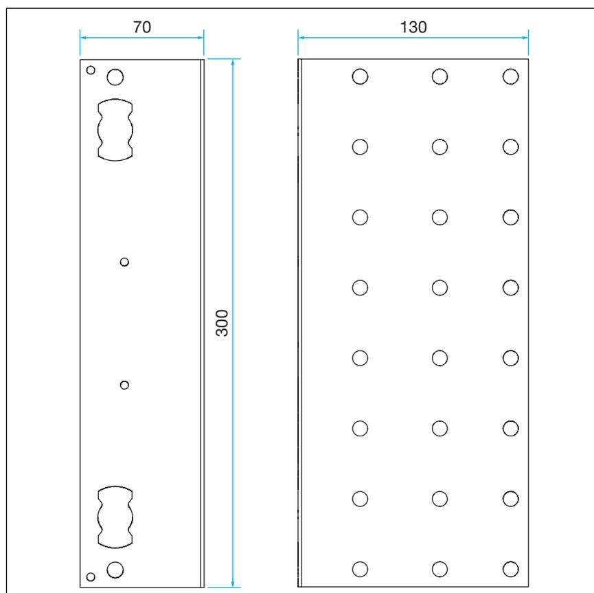
Fig. 2: Installation dimensions
