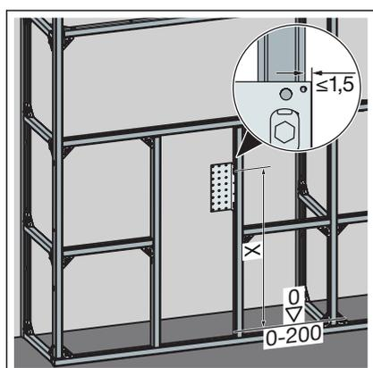
➤ Set the height of the fitting holder according to the information of the sanitary item manufacturer.
