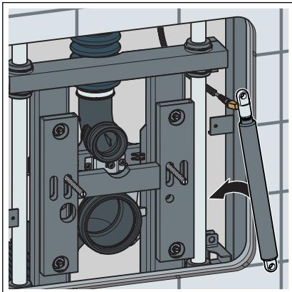
► Insert the new gas pressure spring.
