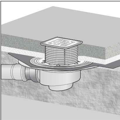
*Fig. 1: General installation example – Floor recess*
