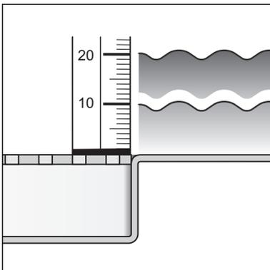
Drainage capacity at an accumulation height of 10 mm above the grate: 0.55 l/s
