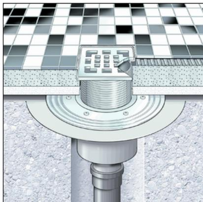
Fig. 3: Construction diagram of a conventional sealing
