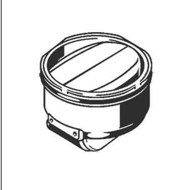
Advantix drains can be equipped with an additional odour barrier, which also closes the drain odour-tight, if the water seal in the odour trap has evaporated. Odour nuisance is even avoided with drains that are only seldom used. Odour barriers can be found in the catalogue.
