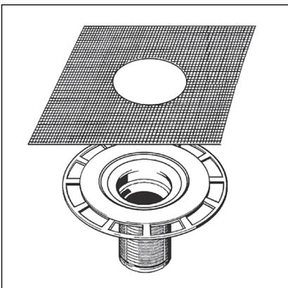
If a bonded sealing is to be applied, a suitable stacking element with sealing collar is required.
