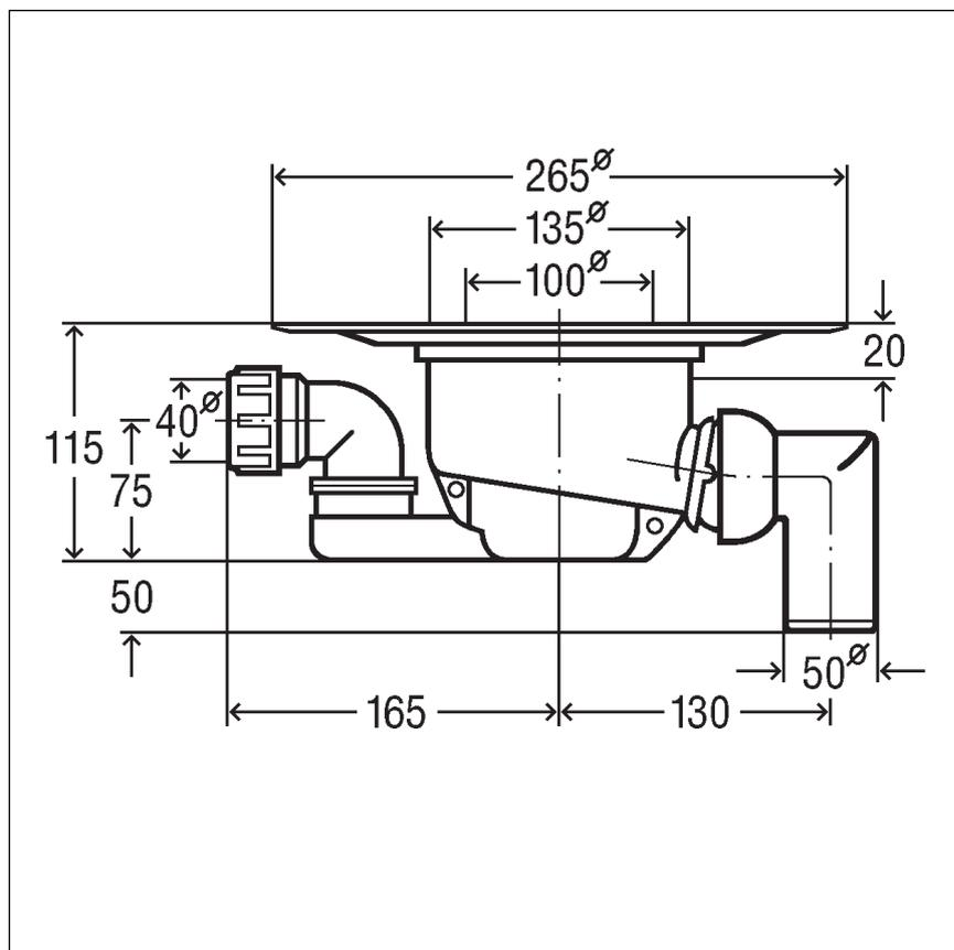
Fig. 7: Dimensional drawing model 4911.65
