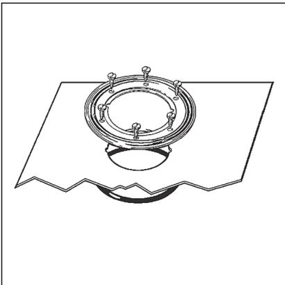
If a conventional sealing is to be made, a suitable sealing collar and a clamping ring will be required.
