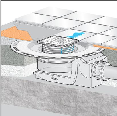
Fig. 2: General mounting example – Mounting on the floor
