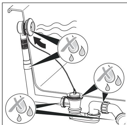
The leakage test is only carried out as a visual inspection.
