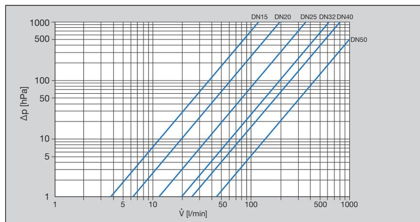
**Fig. 1: Performance diagram slanted seat valve press/threaded connection**
